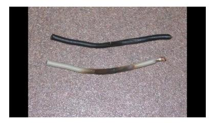
[2m:19s] In order to avoid these types of failures, it is important to have a solid understanding of what the ampacity rating of electrical conductors actually are.
