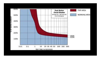
[2m:59s] This graphical representation looks at two separate pieces of data to provide us with the information needed to understand when a given breaker will trip. The first piece of information is time.
