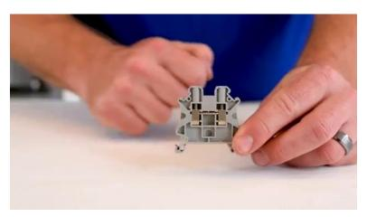
[2m:44s] However, without the ability to provide any fused protection, the pass through terminal block is the most commonly used as a junction point.
