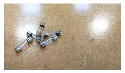
[2m:55s] Using a fuse to both protect and isolate your signals is an inexpensive way to provide the operators with the flexibility they need to troubleshoot equipment without affecting everything in the panel.
