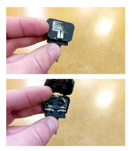
[3m:49s] It is also important to make sure that your fuses are sized correctly for the devices that they are intended to protect.
