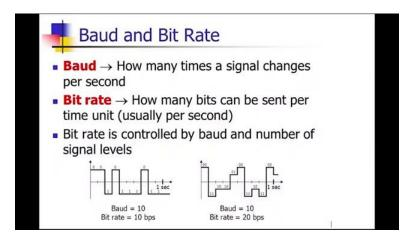
[2m:22s] which simply increases the number of the bits that can be transmitted per second. This is one of the reasons serial communication methods have remained
