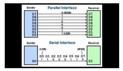
[1m:40s] by which multiple bits can be sent and received simultaneously over multiple communication lines in a single bus or cable. While it may seem that parallel communication would be the preferred method in most cases, this is not true in many situations. Because of the increased complexity and data transmission, it is common to find that it is serial communication that is being clocked at faster speeds than parallel communication buses.
