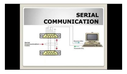
[1m:32s] This means the data will be transmitted just one bit at a time.
