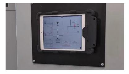
[3m:24s] However, many HMIs can provide remote interface through a cellular device or tablet,
