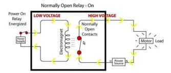
[0m:47s] So, it is important to note that when we have power on the coil, we also have power on the contact side of the relay. When power is removed from the coil, the contacts open and we no longer have power passing through. So, now let's talk about a normally closed contact. So, with a normally closed relay, as you can see, with no power applied to the coil, we have power running through the contact side of the relay. So, when we apply energy to the coil.
