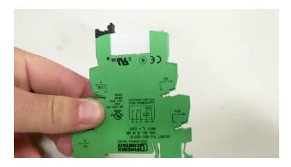
[2m:41s] The internal circuitry of a solid state relay is far more complex than an EMR, but one of the main takeaways that you should remember is that in a solid state relay, there are no physical moving parts.
