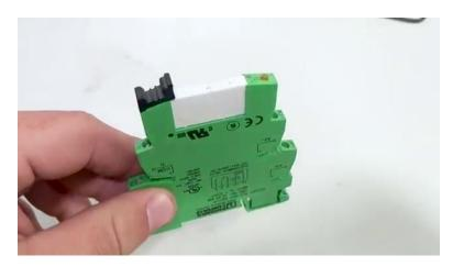
[2m:27s] So when this is activated, the input optical signal will act as the switch, then allowing the higher voltage signal to pass through the relays output components.
