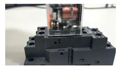
[1m:43s] This movement is made possible by an electromagnet. When power is applied to this magnet, it will act on the movable contact causing the relay to switch. In an EMR it is common to hear the switching sound that is represented by a clicking noise. This audible noise can be helpful when determining the functionality of the relay.
