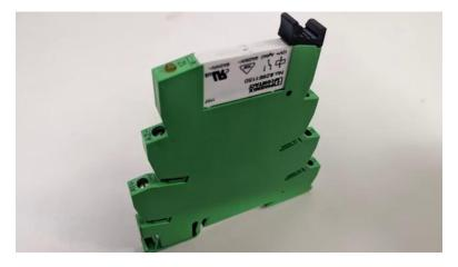
[2m:13s] A solid state relay will use a low power electrical signal to generate an optical semiconductor signal.
