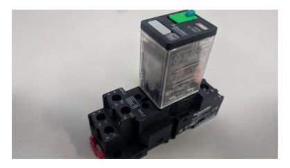
[1m:33s] These moving parts include the contacts that switch between normally open and normally closed stationary contacts in the relay.
