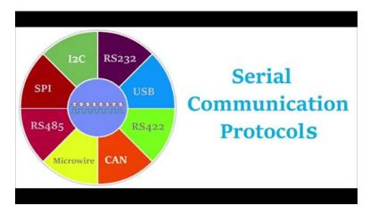
[1m:3s] RS 485 was developed as a replacement or upgrade to the RS 232 standard as well as RS 422,
