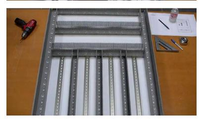
[3m:23s] It is imperative that you account for the wires that will be installed once the panel is located in the field.
