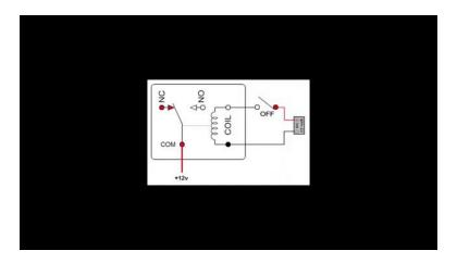
[2m:24s] This state change typically occurs when power is applied to the coil on the relay or other electrical device.
