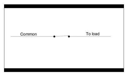
[3m:29s] It is only when the relay or other electrical device is energized or changes state that the normally closed contact will open, thus cutting off the flow of electricity.
