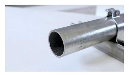
[4m:16s] Once the pole has been secured into the ground, you can simply use some struck clamps that are designed for use with the size of conduit that you are using.
