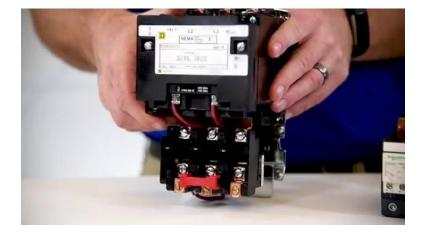
[2m:59s] Lastly, commonly used with motor starters, are motor circuit protectors. These are essentially circuit breakers that are specifically designed to be used with motor starters. They operate by preventing large spikes in current that might be caused from a short circuit.
