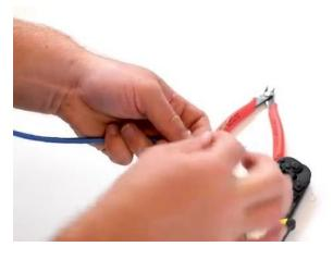
[2m:16s] And at this point, you can see I've exposed the four different pairs of wires within this network cable.
