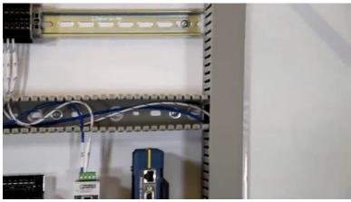
[3m:17s] So make sure to really take time and think about the amount of conductors that will be used, and then ensure that you have enough room to accommodate those conductors with room to spare.
