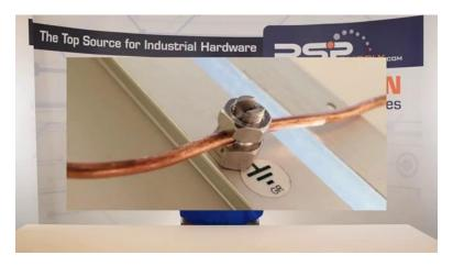
[4m:44s] This energy needs to be dissipated, but because there is no path to ground, the device will retain this energy until it finds a path to ground.
